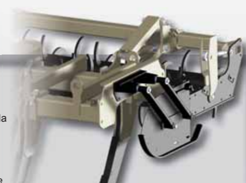
Clod-restricting side boards , a device keeping the clods within the working width of the implement and preventing them from discharging on the already tilled soil or on the soil still to be tilled.
