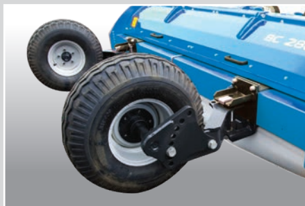
Ruote sterzanti: 10.0/80-12 Steering wheels: 10.0/80-12 Ruedas semigratorias: 10.0/80-12
